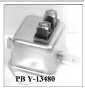
**PB414** clockwork panel mounted indicator switch (suitable for 6, 12 or 24 volt systems), make and break contacts for approx 20-25 seconds then self cancels. body size approx 45mm x 55mm x 25mm. easy to connect input (fused) and exit terminals
