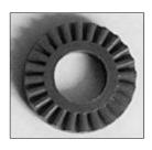
**PB446** gunmetal Simms couplings, unmachined central drive hole available 14 or 15 teeth (48mm diameter), 19 or 20 teeth (57mm diameter) or 23 or 24 teeth (65mm diameter) **PB449** vernier coupling, small size 14/15 teeth, 48mm diameter. made to original pattern in hard rubber
