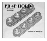
**PB 4P HOLD** spare spark plug holder in cast aluminium, supplied tapped but not polished. size approx 115mm x 25mm, available for the 18mm or 14mm plug sizes **PB 6 HOLD** spare spark plug holder in cast aluminium, supplied tapped but not polished, size approx 130mm x 67mm. available for the 18mm, 14mm or 10mm plug sizes. **PB452** spark plug adaptor allows a 14mm plug to be fitted in to a 18mm plug hole, enabling user to take advantage of the wider heat range of 14mm plugs
